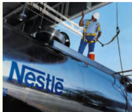
Work-place safety: a worker at Ocotlán, Mexico, wears a safety harness to inspect and clean a milk tanker
